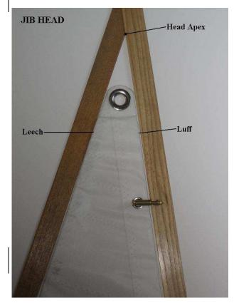
**NOTE:** On the girth measurement, be sure to use the head apex when matching up to the tack and clew. Do not measure cringle to cringle as this will incorrectly increase your girth measurement. Refer to the photos at left and below, 4a-c.
