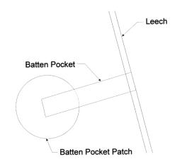
8.6 Flutter patch covers at seam to reinforce the sail edge are permitted. This lessens "comb-out" of the seam and greatly reduces the chance of seam failure at the leech.
